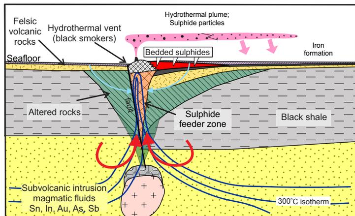
**Figure 3.** Model for the formation of volcanogenic massive sulphide (VMS) deposits. Modified from Goodfellow (2007).
