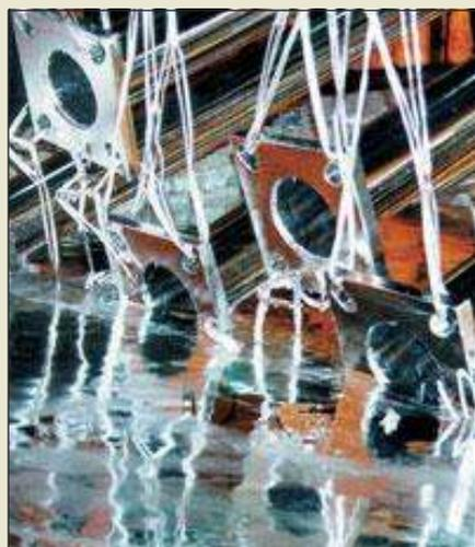
Hot-dip galvanization where steel parts are dipped in liquid zinc (bottom of photograph) to prevent corrosion of the steel.
