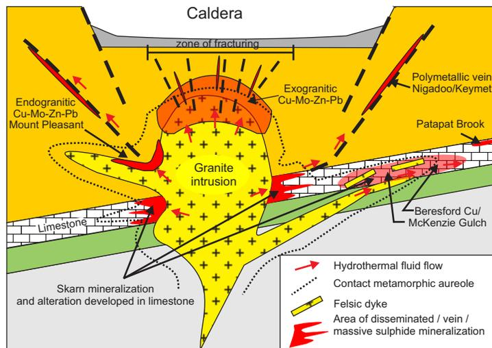
**Figure 4.** Model relating endogranitic, polymetallic vein, and skarn zinc mineralization to granitic intrusions with examples cited in text. Note that a significant example of an exogranitic zinc deposit has not been identified in New Brunswick.
