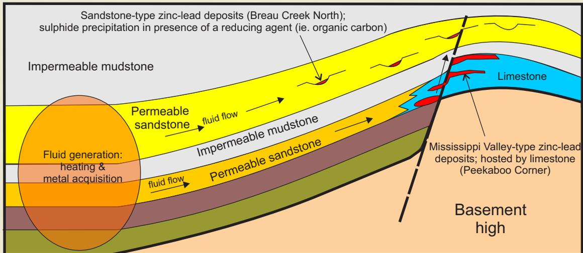
**Figure 5.** Conceptual model for the generation of sandstone-type and Mississippi Valley-type zinc-lead deposits, with New Brunswick examples. Compiled from Graves and Hein (1994), NBDEM (2013), and Sangster (1996a and b).
